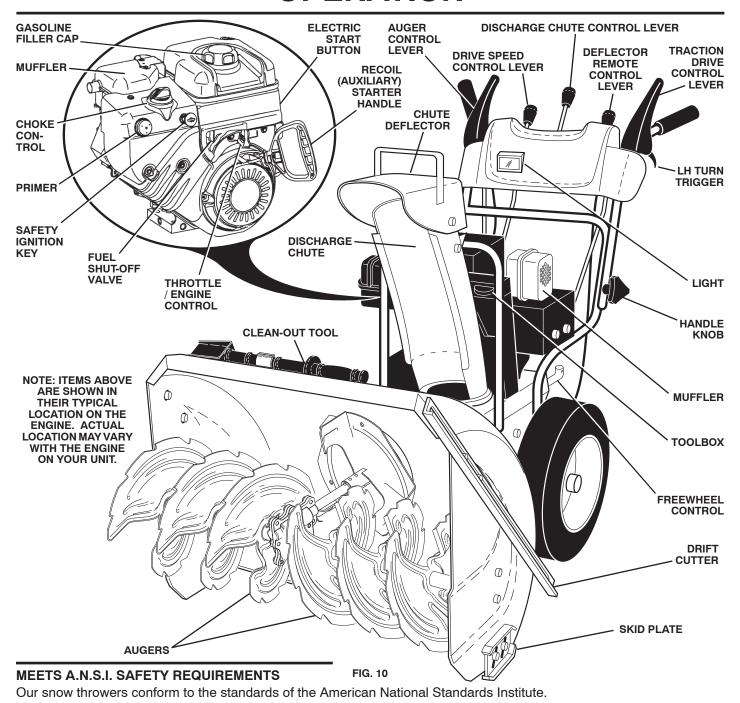
**Toolbox -** used to store spare shear bolts, locknuts and wrench.
